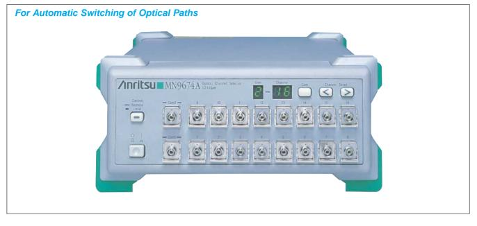
The optical channel selector is a switching device used for outputting the light that is inputted to the common channels to any channel. The above devices are equipped with eight (for MN9662A/9672A) and sixteen (for MN9664A/9674A) channels, making them ideal for the evaluation of devices for WDM and various optical transmission devices<sup>\*</sup>.
